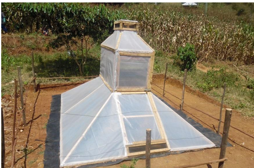
A family solar dryer puts the sun's rays to work to preserve the vegetable harvest.
