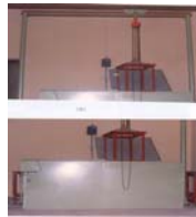
d). Pasteurizer (hot water Tank; carriage System and Crate containers
