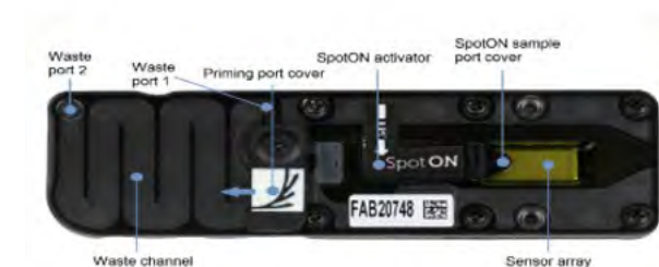
Figure 1: (right) The MK1c unit (size: h33 x l142 x w118 mm) currently on hire from Taiwan Nanopore and (left) an annotated picture of the MinION flow cell that fits inside the MK1c.
