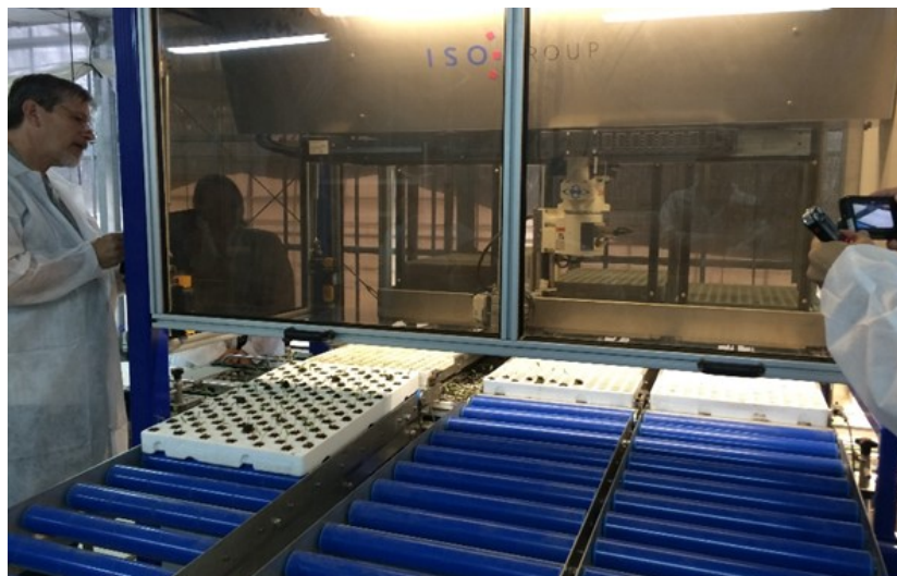
Figure 1. A sorting machine that creates uniform stands of seedlings in each tray. (Photo by Chieri Kubota)
