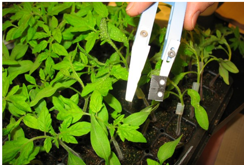
Figure 4. A grafting cutter is designed to cut plants in the tray at a consistent angle.
