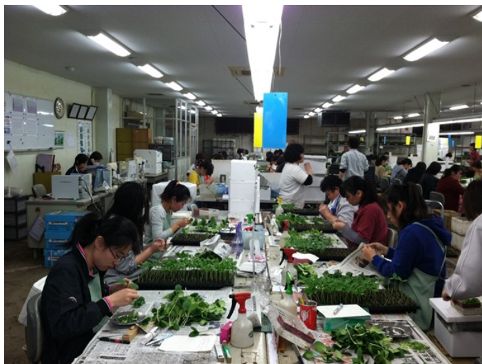
Figure 1. An example of a cellular workflow design in a grafting nursery where each worker performs all the steps of “assembling” grafted plants.
