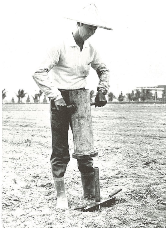
Extracting soil samples to assess the fertilizer residues left behind by an earlier crop of Chinese cabbage.
