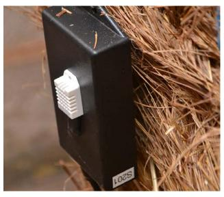
Data-logging sensor attached to a vegetable cooling device. Photo by Lauren McKown, MIT D-Lab.
