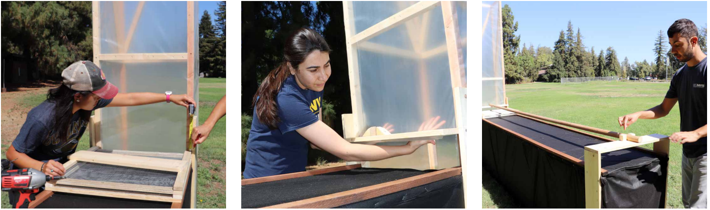
Photos from left: Build a shelf at each end of the drying table. Cut a rectangular window into the chimney plastic and attach edge of the plastic to the shelf. Place bamboo or wood pole across the top of the shelf, which will hold plastic above trays when in use.
