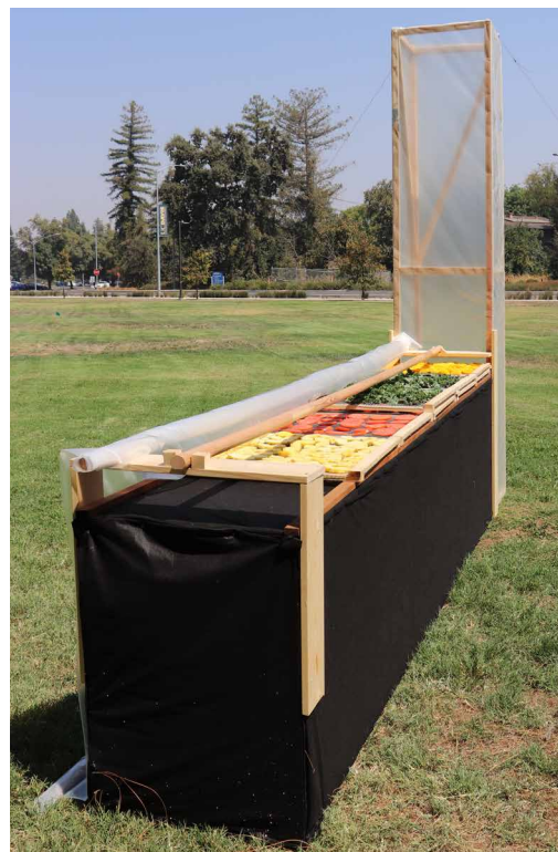
Built with widely available materials, the chimney solar dryer combines a table for drying fruits and vegetables with a chimney.
