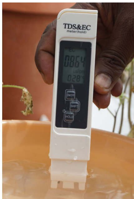
Figure 39: Measuring EC of the medium
