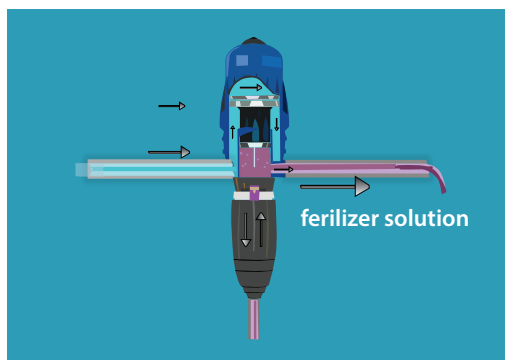
Figure 30: Blended solution is discharged into the water line
