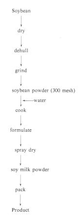
Fig. 5 Flow sheet of instant soy milk powder production (II).
