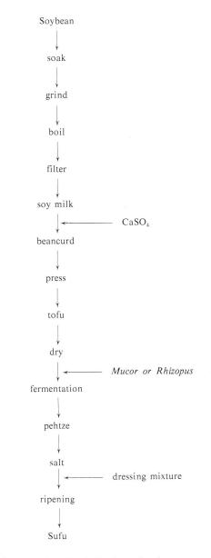
Fig. 9 Flow sheet of sufu production.
