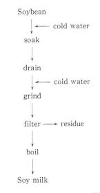
Fig. 1 Flow sheet of soy milk production by traditional method.
