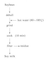
Fig. 2 Flow sheet of soy milk production by Cornell method.
