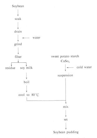
Fig. 6 Flow sheet of soybean pudding production.
