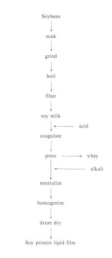
Fig. 8 Flow sheet of soy protein lipid film by drum drying.
