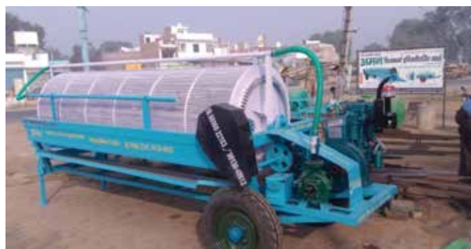
Carrot cleaning machines developed by a 6 th grade-educated mechanic in Bahawalpur village of Hisar district (top & below)
