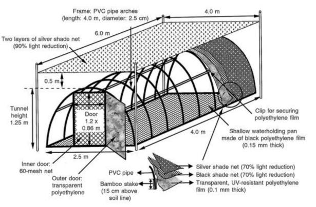
Figure A. Technical drawing of grafting healing chamber
