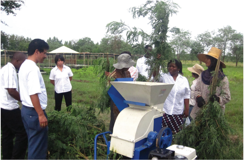
Figure 6. Chopping compost materials using a motorized shredder.
