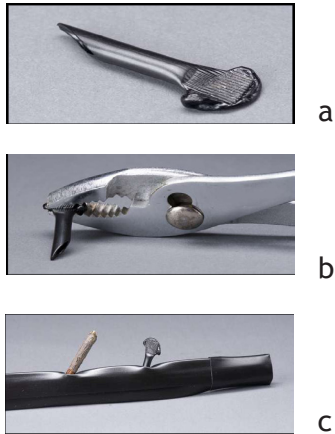
Figure 23. Heated tubing (a) crimped with pliers (b) and inserted or plugged in drip tape hole (c)
