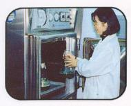
20 Autoclave the juice (120°C, 1.05 kg/cm<sup>2</sup> for 20 minutes).
