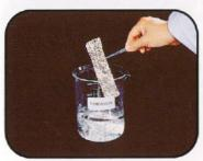
27 Dip oviposited foil (foil on which eggs have been laid) in 10% formalin for 30 minutes and then rinse the foil in running tap water for 15 minutes to completely wash off the formalin disinfectant.
