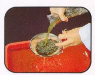
**21** Filter the autoclaved juice through an ordinary sieve and discard plant debris.
