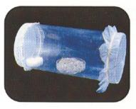
41 Place 100 *Oomyzus* pupae in a small petri dish inside a 15-cm diameter, 30-cm long acrylic or plastic cylinder. Also place absorbent cotton soaked in honey solution in a small petri dish inside the cylinder. *Oomyzus* adults emerging from pupae will feed on the solution. *Oomyzus* rearing can be done at the same temperature as for *Cotesia*, 26-28°C.
